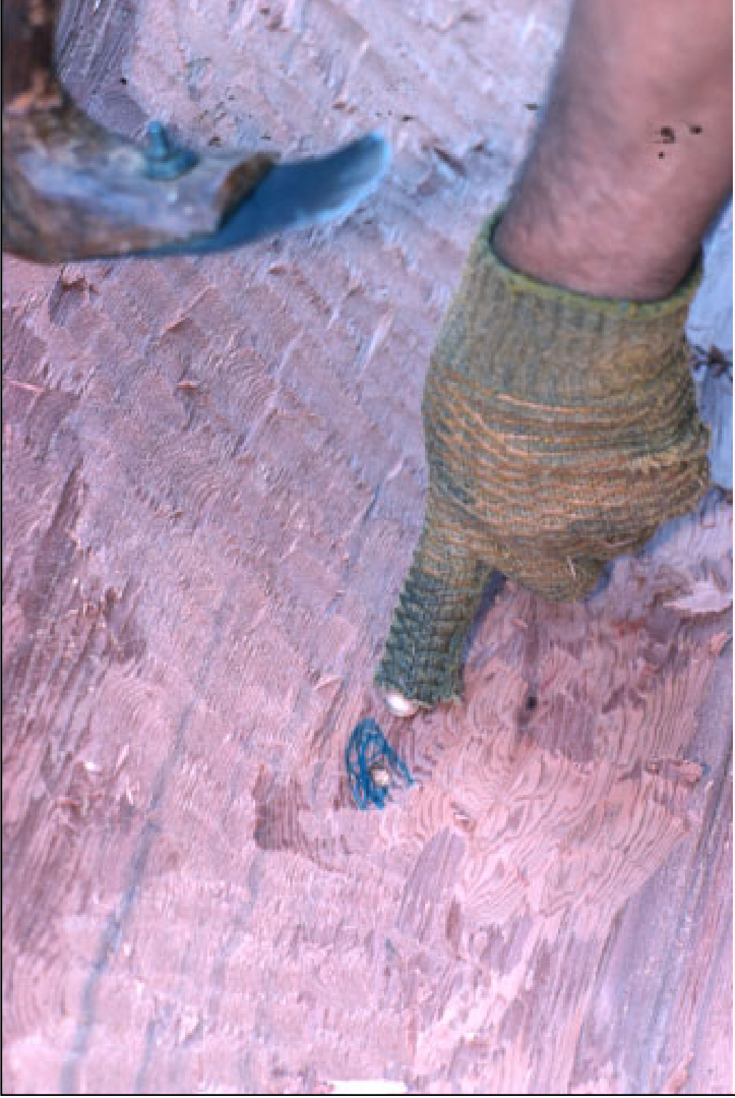
Pegs of a premeasured size help the carvers to achieve the correct thickness for the canoe's sides and bottom.
